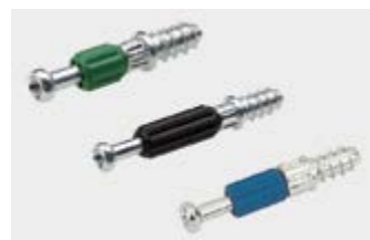
Coloured plastic sleeves in easy-to-grip fluted design indicate dowel lengths. Green (dowel length 20 mm) for Rastex 15, blue (dowel length 24.5 mm) for Rastex 25 and black (dowel length 30 mm) for Rastex 15.
