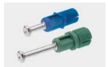
Fast, tool-less installation, simply press by hand into the drilling in the carcass side. Easy to tell apart with coloured expanding elements for 8 mm (blue) and 10 mm (green) drillings.
